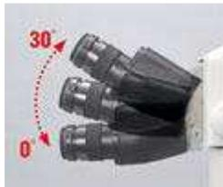
The AZ100 comes standard with eyepiece tubes that tilt from 0° to 30°. This feature enables the optimal eye level for the observer's height and posture as well as the sample height. Two different beam-split ratios for the binocular and photo port can be selected: 100:0/0:100, which is suitable for photo documentation; or 100:0/20:80, which enables visual observation while displaying an image on a monitor.
