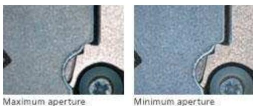
The AZ100 ships complete with an aperture stop that is effective not only for visual observation, but also for the capture of digital images. This aperture stop allows you to freely change contrast and field depth based on your specimen requirements.
